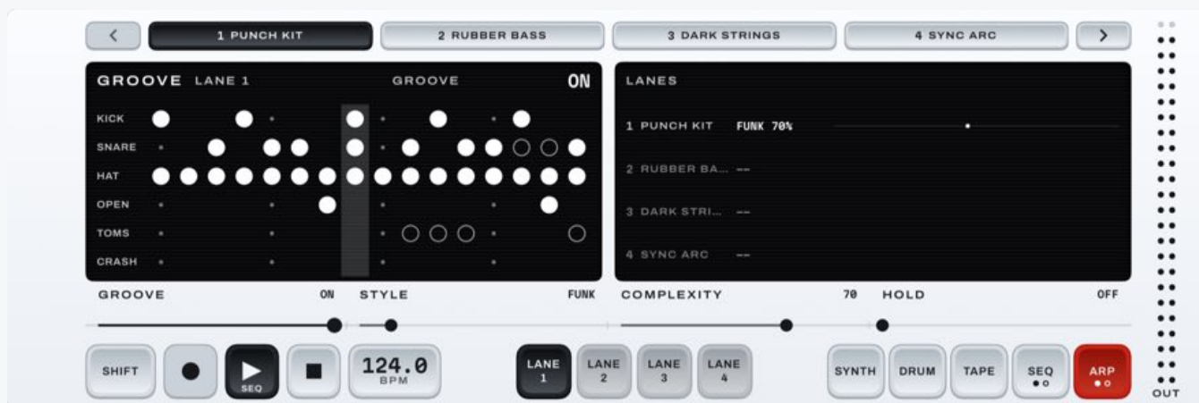
Figure 6.2 A groove in its fill bar. The shaded column is the sixteenth playing now; the hollow dots are hits that join higher up COMPLEXITY.
