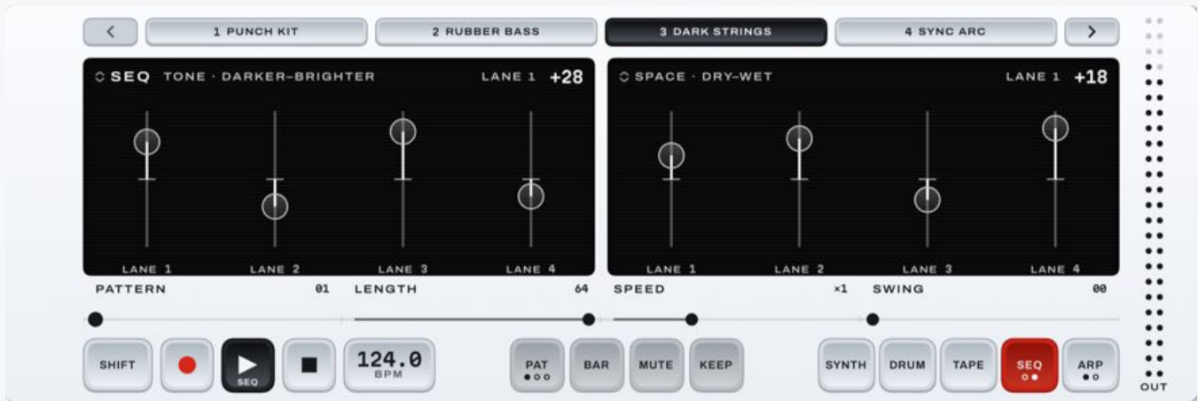
Figure 6.3 TONE on the left, SPACE on the right. The bright line shows how far each lane is from its saved sound.
