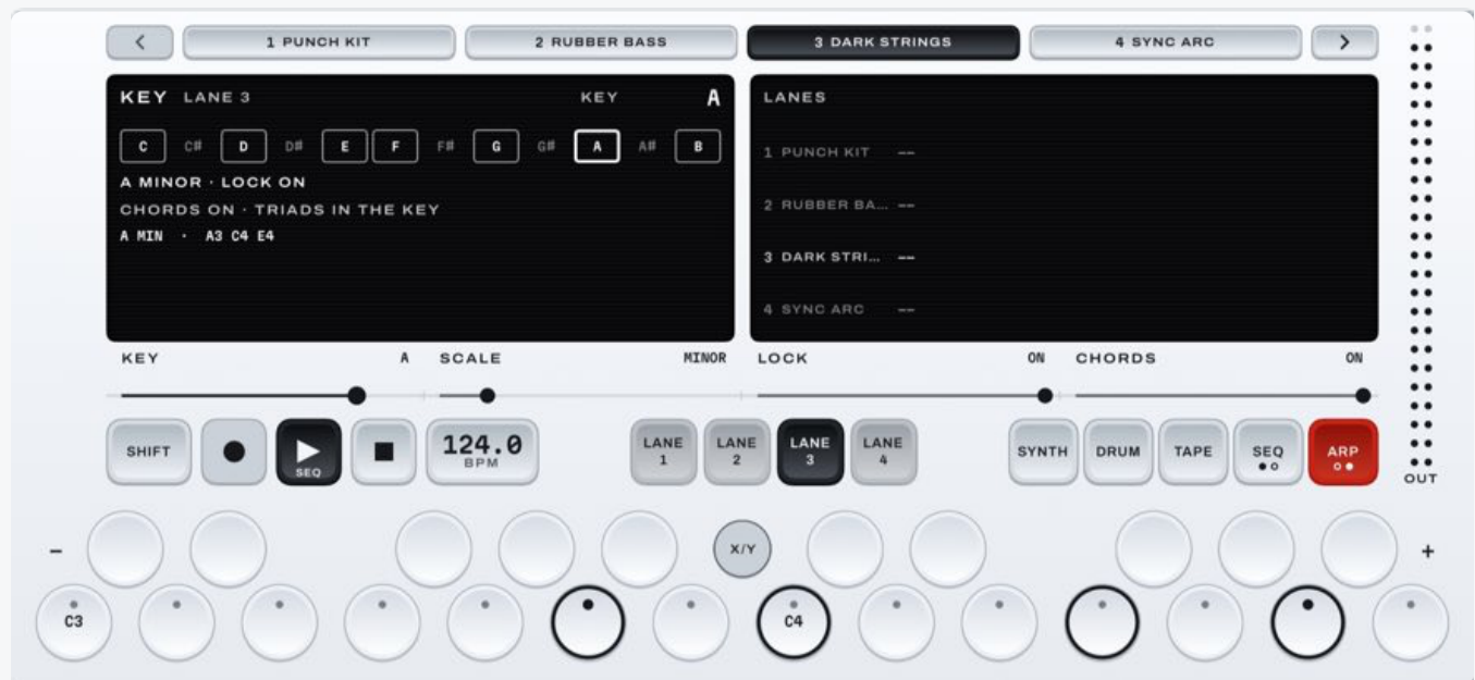
Figure 5.1 KEY on A minor, with LOCK and CHORDS on: the window names the scale, and the chord the last key played.
