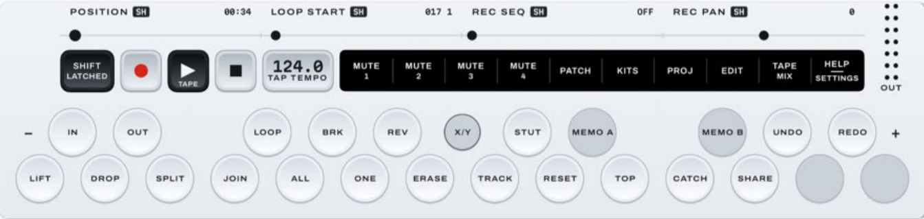
Figure 7.3 TAPE under SHIFT: the keyboard is the tool row, and the strip starts with each track's MUTE.
