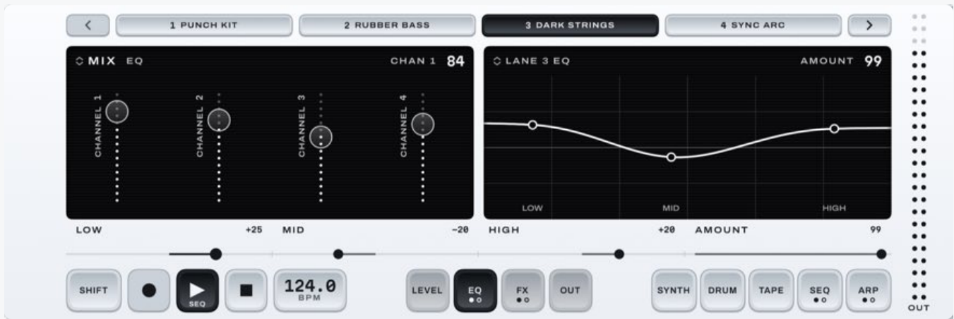
Figure 8.2 Lane 3's own EQ: the curve and the band change that lane alone.
