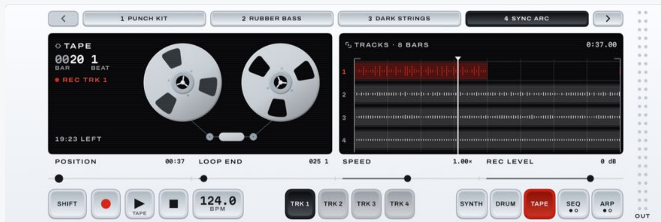
Figure 7.1 A song on tape. The filled track key, TRK 1, is where the next take goes, so its row is drawn red.
