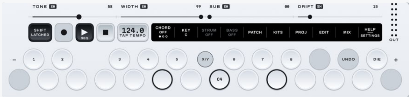
Figure 1.3 SHIFT latched on SYNTH: the strip starts with SYNTH's chord buttons, then the doors and HELP / SETTINGS. The top row of keys is now the quick slots.
