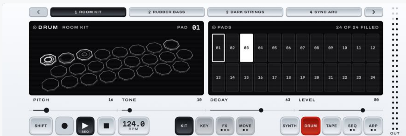
Figure 2.3 The KIT page: the band edits pad 01, the brightest plate and the outlined pad. Pad 03 is lit because it is sounding.
