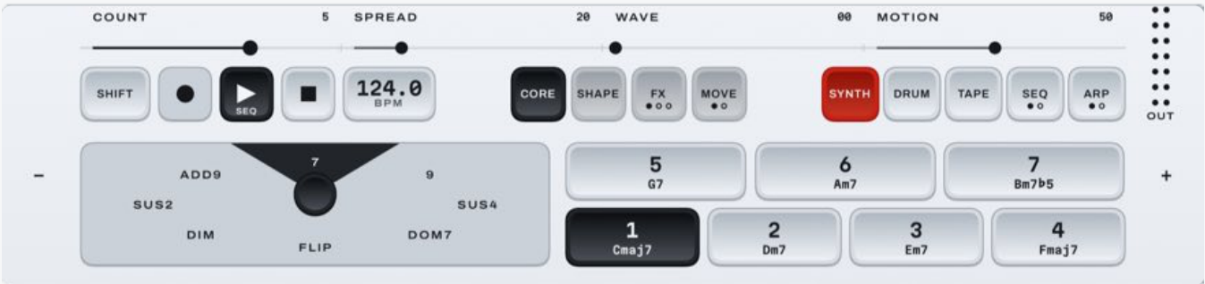
Figure 5.2 Chord 1 with the stick pushed up: Cmaj7, and every key shows its seventh chord before you press it.
